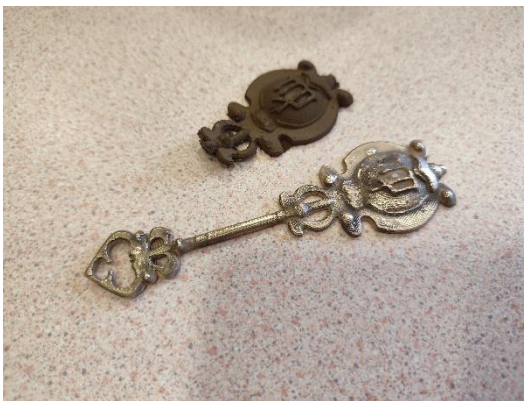
3D printed demonstrators in Bronze: (brown) printed, bright (printed, debinded and sintered)
