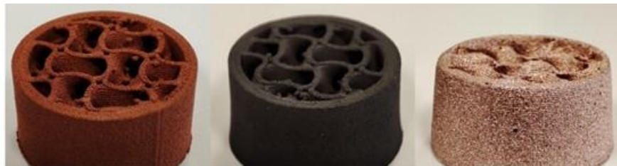
Copper structured reactor, (a) printed, (b) debinded and (c) sintered
