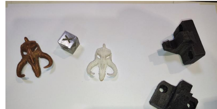
Filament 3D printed demonstrators in (from left to right) Copper, 316L stainless steel, Zirconia, PA6-CF.
